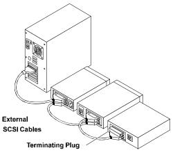
Figure 1-11. Terminating the Last External SCSI Device
